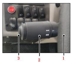
Steering wheel 2. Gear switch 3. Horn
