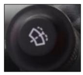
Fig.3.2.9 Front windshield spray switch
