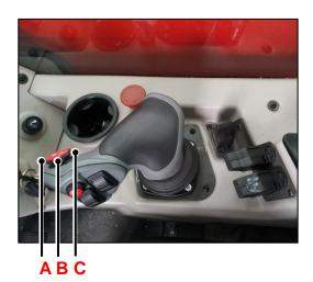
Fig.3.2.15 D Gear/N Gear/R Gear
